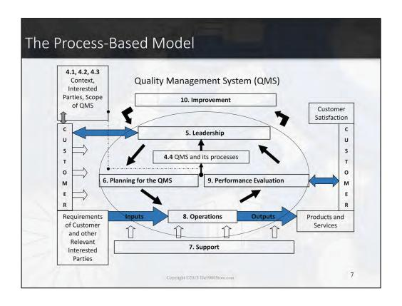
This example of the process-based model is similar to the one included in the standard (Figure 1).
